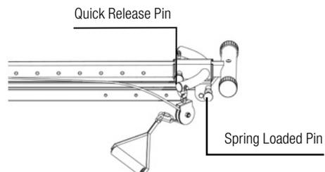
B. Take hold of the Vertical Column and pull it up until it is upright. Release the Spring Loaded Pin. You should hear it lock back into place. (**NOTE:** pin shown in picture is on right side)
