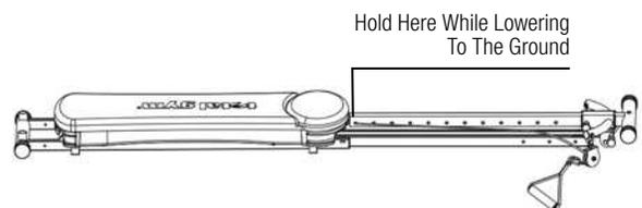
5. **A.** Next remove plastic packing ties from the top and bottom of the Vertical Column. Pull out the Spring Loaded Pin Knob located at the left rail (**NOTE:** pin shown in picture is on right side) to release Spring Loaded Pin. Continue to hold pin out while performing the next step.
