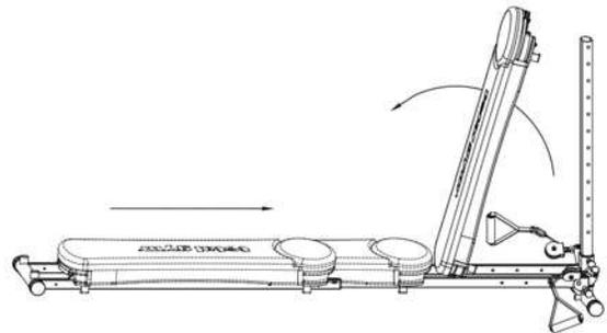
3. Next, pull the Spring Loaded Pin to release the Rail and fold the exerciser together as shown in Fig. 7B. Be sure you release the Spring Loaded Pin before folding.
