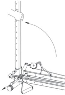
**IMPORTANT:** Be sure the Spring Loaded Pin is locked into place before using your unit. You will know the pin is locked into place when you can see the end protrude through the inside of the rail bracket.
