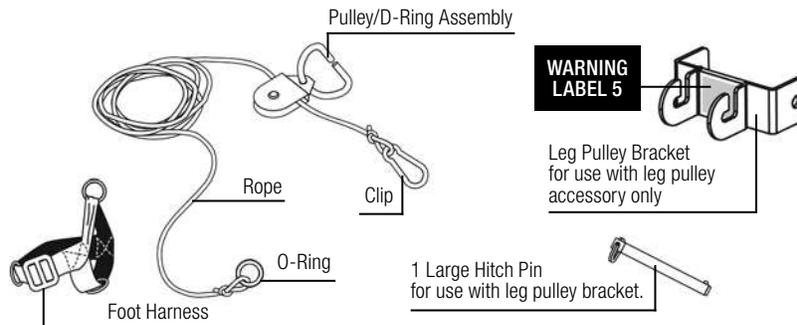
1. Connect the Leg Pulley Bracket to the top of the Vertical Column by aligning Bracket with the hole at the top of the column; be sure bracket is right side up. Insert Large Hitch Pin through the hole to secure Bracket onto the Vertical Column.
