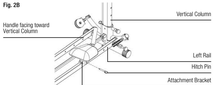
3. Insert the M8 x 60mm Hitch Pin through the holes on the Attachment Brackets and through the hole on the Left Rail as indicated by arrow.
