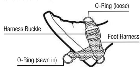
2. Detach the Cable Assembly from the hook on the underside of the glideboard and attach O-Ring from the Leg Pulley Assembly.
